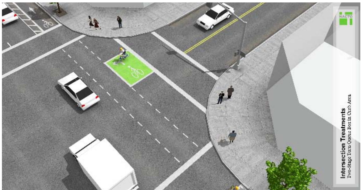
Intersection Treatments Two-Stage Turn Queue Box in Parking Lane Adjacent to Bike Lane
