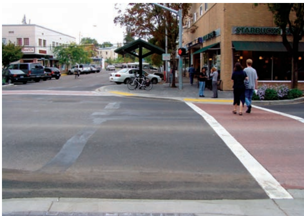
Curb extension provides room for bike parking
