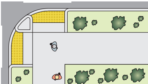
Figure 4-32: Ramp placement, sidewalk with furniture zone
