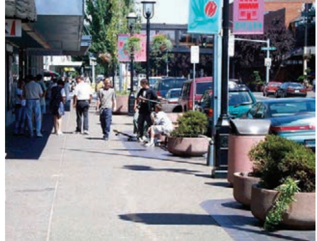
A well organized furniture zone leaves the pedestrian zone clear of obstacles
