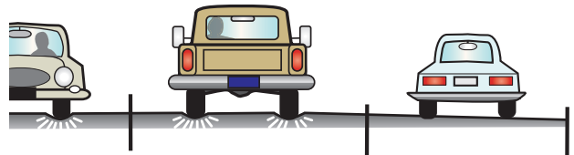
Figure 2-9: Motor vehicle travel lane offset by bike lane results in larger effective turn radius
