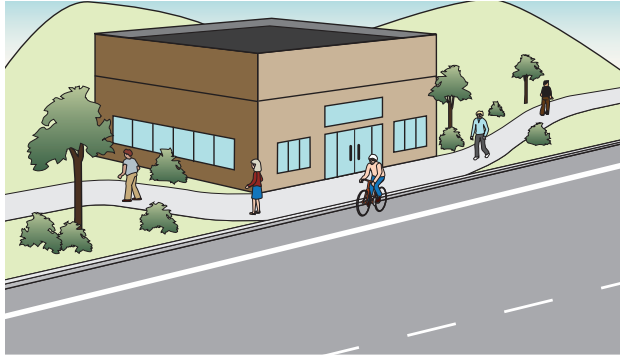
Figure 4-6: The furniture zone may be eliminated or reduced at pinch points
