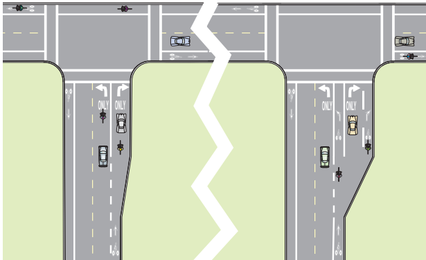
Figure 6-7: Bike lane at T-intersection
