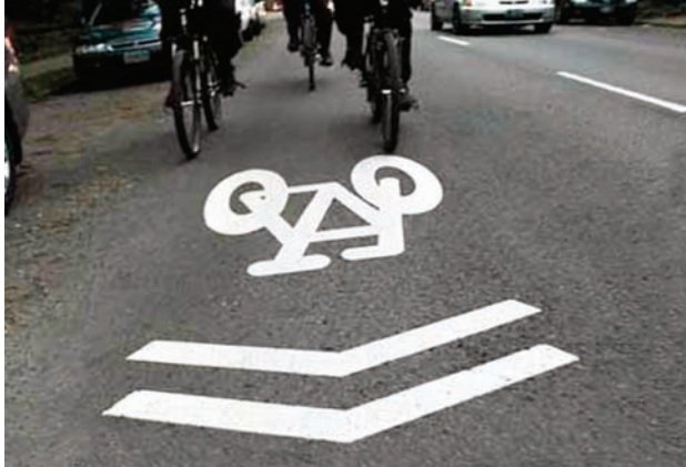
Sharrows indicate where bicyclists should position themselves in the roadway
