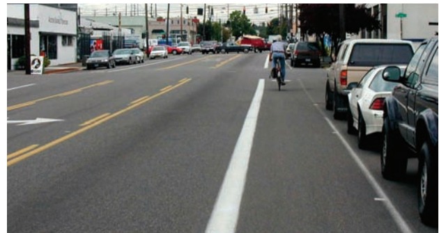
Typical bike lane on urban higher speed/volume roadway
