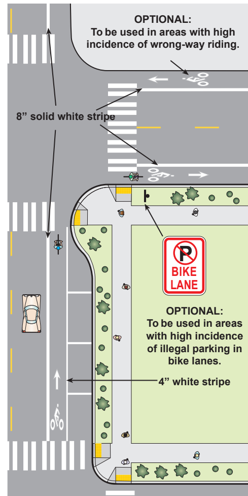
Figure 1-26: Oregon standard bike lane marking
