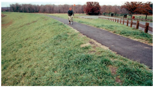
Gentle grassy slope eliminates the need for railing
