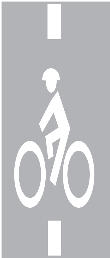
Figure 1-34: Bike symbol for loop detection placement
