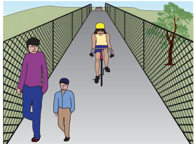
Figure 7-10: High fencing at path edges creates cattle chute effect
