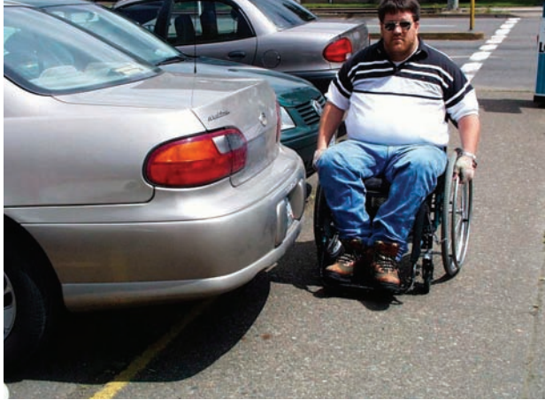
Wheel stops prevent sidewalk encroachment
