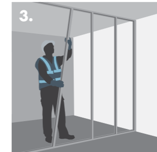
3. Twisting Knauf Acoustic 'C' Studs into position.
