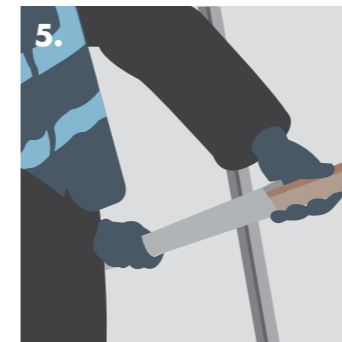
5. Insert timber battens within Knauf 'C' Studs to provide fixing for door frame (if required).
