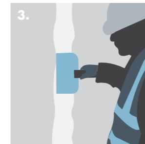
3. Applying Knauf Joint Cement Easy Sand over the tape.
