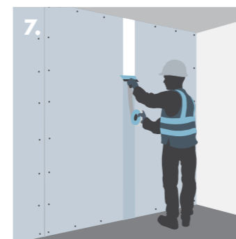
7. Taping and jointing for a seamless finish.
