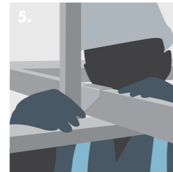
5. Adjusting the Knauf MF Ceiling Channel.
