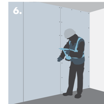
6. Stagger the boards, to ensure all joints overlap.
