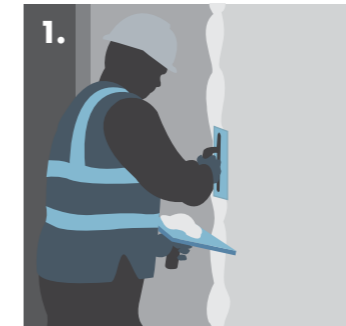
1. Applying a continuous band of Knauf Plasterboard Adhesive around the perimeter.
