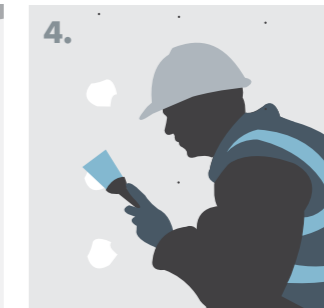
4. Covering screw heads with Knauf Aquapanel Joint Filler – Grey.
