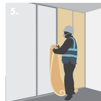
5. Inserting Knauf insulation quilt between the Knauf 'C' or 'I' Studs.
