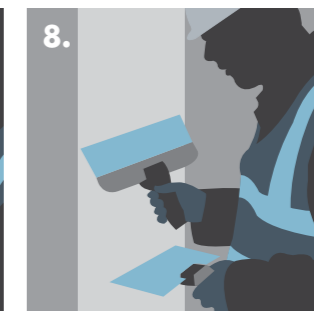
8. Tape and joint for a seamless finish.
