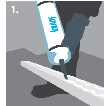
1. Applying continuous beads of Knauf Sealant to perimeter framing.
