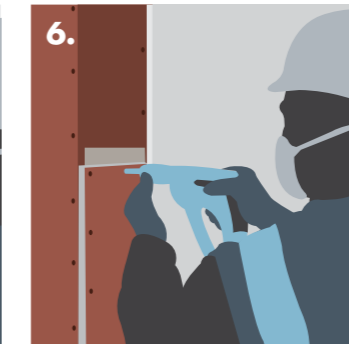
6. Fixing outer layer of Knauf Fire Panel.
