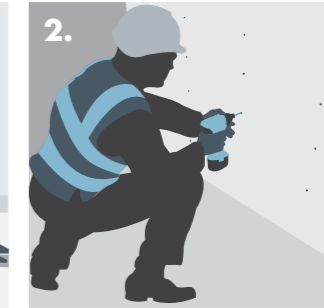
2. Fixing the boards to the background members.
