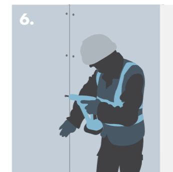
6. Fixing Knauf Soundshield Plus to the frame.
