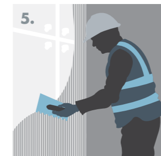
5. Applying notches within the basecoat.
