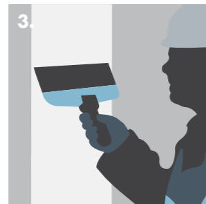
3. Applying first coat of Knauf Joint Cement Easy Sand.
