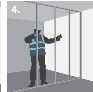
4. Positioning studs at 900mm centres.
